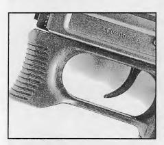
Operators should grasp the MP9's unique abbreviated foregrip with their thumbs looped through the trigger guard in the same manner as used on the Beretta 93R machine pistol.
